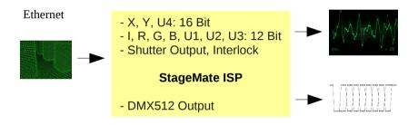
The converter implements a preliminary version of IDN, the ILDA Digital Network protocol currently under development. In addition to streams of frames, the converter can process streams of samples – and thus precisely synthesize analog waveforms simultaneously on any of its outputs.
