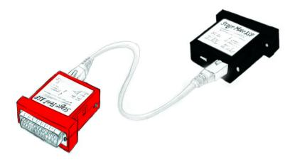
This mode is used as a direct substitute for the ILDA ISP-DB25 and ISP-DMX cables used with most laser projectors. Both converters (StageFeed ISP and StageMate ISP) are connected directly to each other via a standard Ethernet patch cable. Cable length should remain within the 100-meter limit of Cat5/Cat5e cabling.
