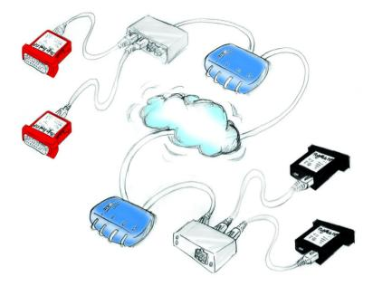
This mode can be used to bridge even larger distances or infrastructures. Since there is no common broadcast domain, StageFeed has no way of identifying its partner using the unique UnitID. Setup is more complicated and IP addresses are the only way of finding the configured StageMate.
